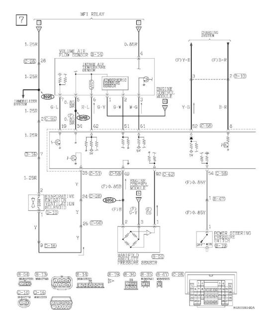
MFI System ((A/T) With Intake Manifold Tuning (IMT) System) Part 7
