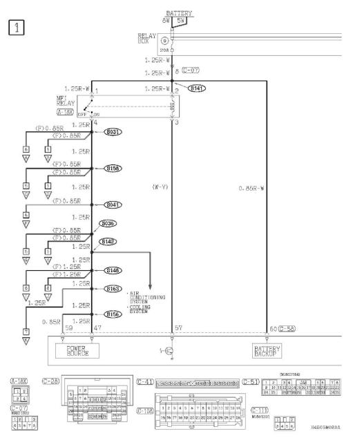
MFI System ((M/T) Without Intake Manifold Tuning (IMT) System) Part 1
